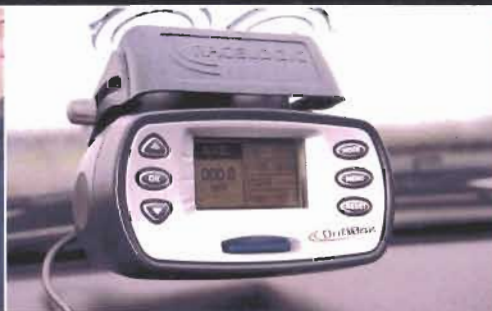
GPS-based data-logging service also allows DriftBox to figure speed and lap times and standing starts
