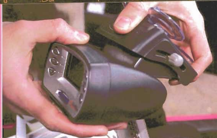
The Racelogic DriftBox is simplicity itself to fit to your car. Simply snap it into the mount, plug in the 12v power source and attach to
