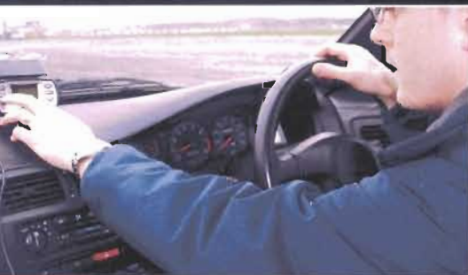
GPS-based data-logging service also allows DriftBox to figure speed and lap times and standing starts
